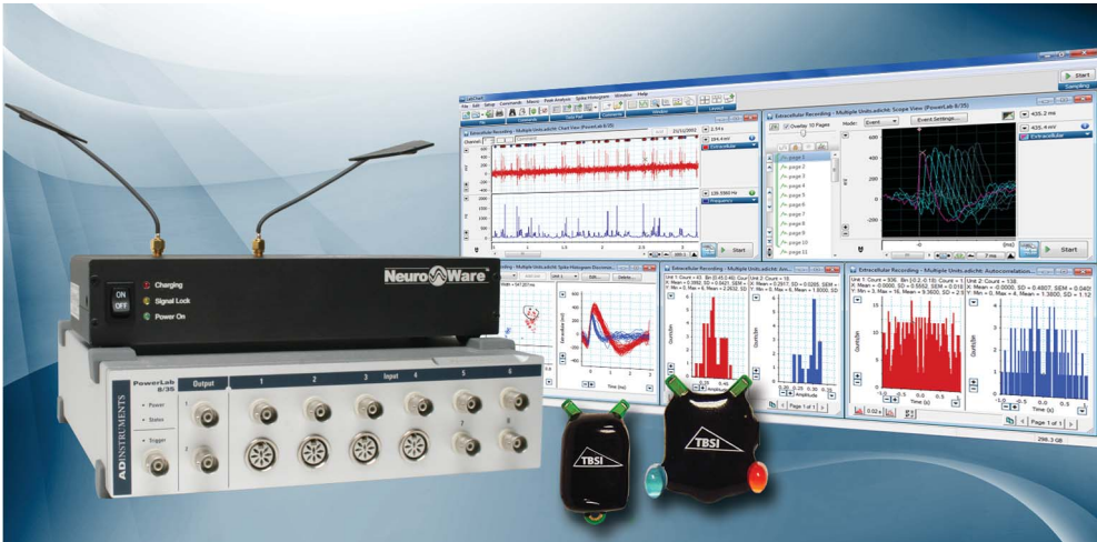
The complete TBSI Wireless Neural Recording Systems feature the PowerLab data acquisition unit, industry-leading TBSI Headstage Transmitter and Headstage Receiver, as well as powerful and flexible LabChart software.
