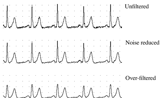
Figure 5. An electrocardiogram (ECG) with various low-pass filter settings: some filtering cleans up noise, but too much distorts the high-frequency spikes.
