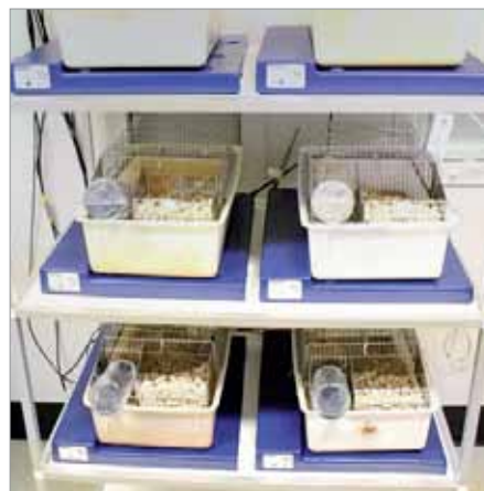
Subjects implanted with telemeters can be housed side-by-side in non-conductive enclosures.
